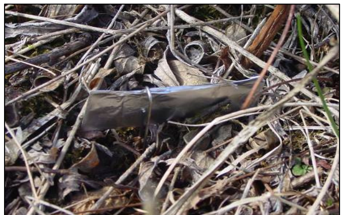
Fig 2. left: Aluminum tag with heat-sensitive paints, melting at 79, 163, 246, 316, 399, and 510°C respectively (from left to right). right: Tag wrapped in foil placed at soil surface prior to burn.
